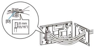
4 Mount the station on the mounting bracket [A].
