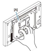
2 Fasten the mounting bracket to the wall with the screws [B] (x2).
